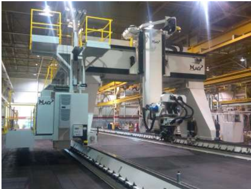
Automated Carbon Fiber Lay-up For Spar Cap Production
